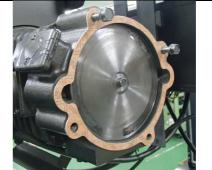
Packing between electromagnetic brake casing and stationary core
