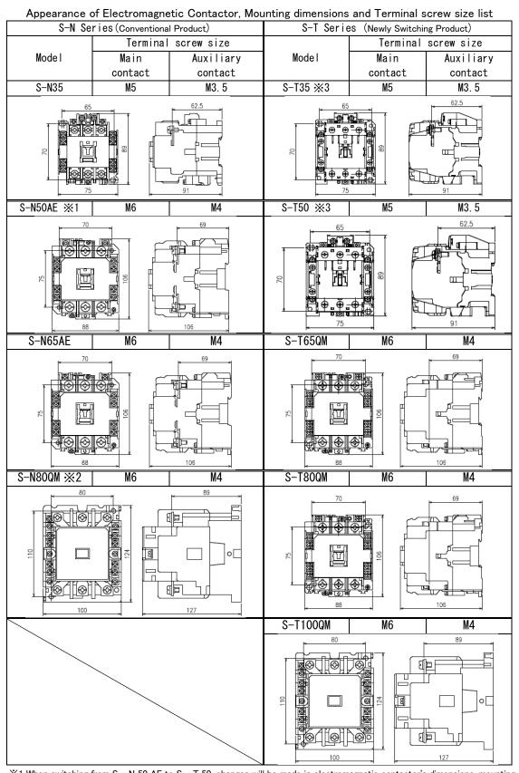
%1 When switching from S - N 50 AE to S - T 50, changes will be made in electromagnetic contactor's dimensions, mounting dimensions.
